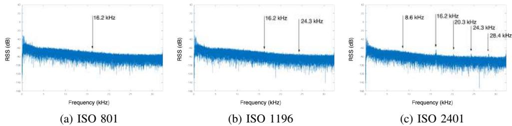
Fig. 8: ISO's effects on frequency distortions for light #3.
