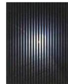
Fig. 2: The rolling shutter effect captured by a Samsung Galaxy S8 over a modulated LED.
