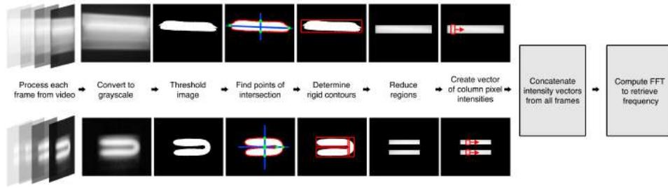
Fig. 6: Image processing algorithm for isolating regions of light.
